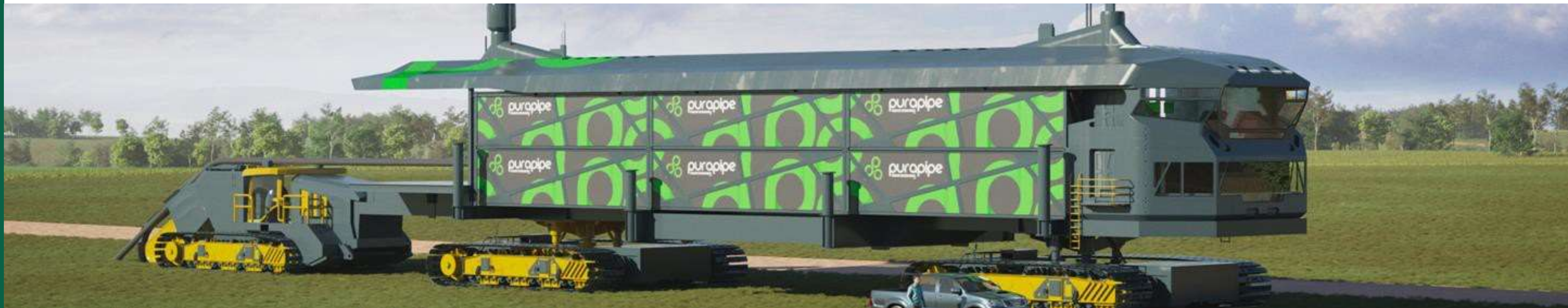
Purapipe Mobile Pipeline Production Unit (MPPU) - artist rendition
