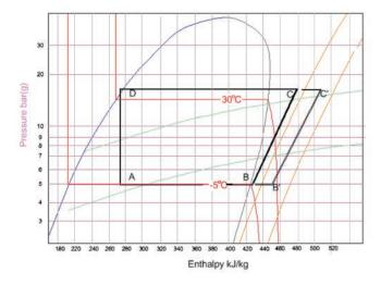
The impact of suction superheat can be seen above. The refrigeration effect stays the same because in most cases the superheating occurs outside the evaporator as the suction line is heated by ambient condition. Superheating that takes place outside the evaporator and provides no useful refrigeration effect is termed un-useful super heat.
