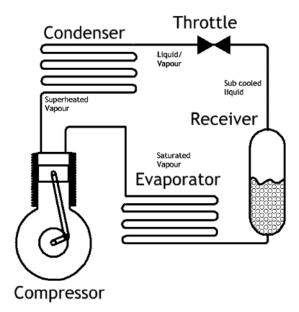
The hot and relatively high-pressure gas is delivered to the condenser (a heat exchange matrix) usually compatible with air or water-cooled condensing temperatures that can be achieved with natural or forced convection and ambient air or water temperatures. In many applications evaporative water-cooling might be employed.
