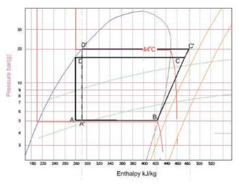
If the same refrigerant were to be used but the condensing temperature is elevated then there is a detrimental effect on the cycle performance. The refrigeration effect is reduced and compressor power is increased.
