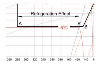
Because the cooling of the refrigerant on expansion is achieved adiabatically, the net enthalpy of the mixture (flash vapour and cooled refrigerant) remains constant and that expansion process is illustrated in the chart opposite by the Line D to A where the enthalpy is considered constant.
