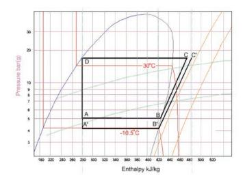
The theoretical coefficient of performance or COP refrigeration effect to power expended can be determined as 139kJ/kg/ 62 kJ/kg or in this case reduces to 2.24.
