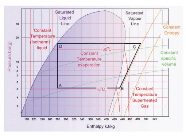
The black bubble line represents the saturated vapour line. All of the refrigerant has evaporated and is a gas. To the right of this line the refrigerant remains a gas and heating at constant pressure results in additional sensible heat and increased temperature and the gas is superheated above the saturation temperature.
