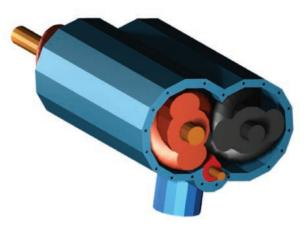
The screw compressor is also a positive displacement machine. Air is drawn in through an intake port and trapped between lobes of two intermeshing screw rotors. The intermeshed volume decreases along the rotor length and the air is progressively compressed until discharge. The rotor length is fixed and thus the compression ratio (Volume Ratio) essentially fixed, regardless of speed. The variation of speed does not change the volume ratio.
