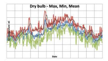
An air cooler (refrigerant to air as opposed to refrigerant to water) will have to operate with a relatively high LMTD (because the heat transfer coefficients are poorer) and will operate with a 12-15°C differential over the dry bulb temperature. Given that a dry air cooler may be designed to operate with 12-15°C differential over the prevailing ambient dry bulb, then for the greater part of the year (>60%) a theoretical condensing temperature of 30°C
