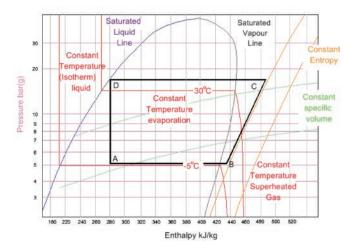
In the diagram above the liquid refrigerant is evaporated from A to B and the enthalpy (energy content) increases.
